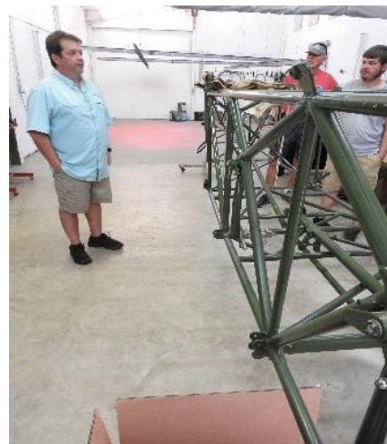
Kevin Kimball talks about the frame of the fuselage that will be part of Kal's plane.
